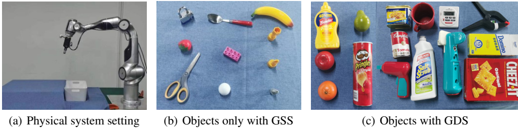
Figure 8: Robot and object settings in the real-world grasping experiments.
