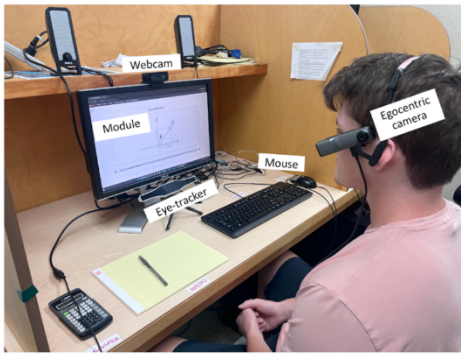
Figure 2: Instruments used for collecting multi-modal data in the study.
