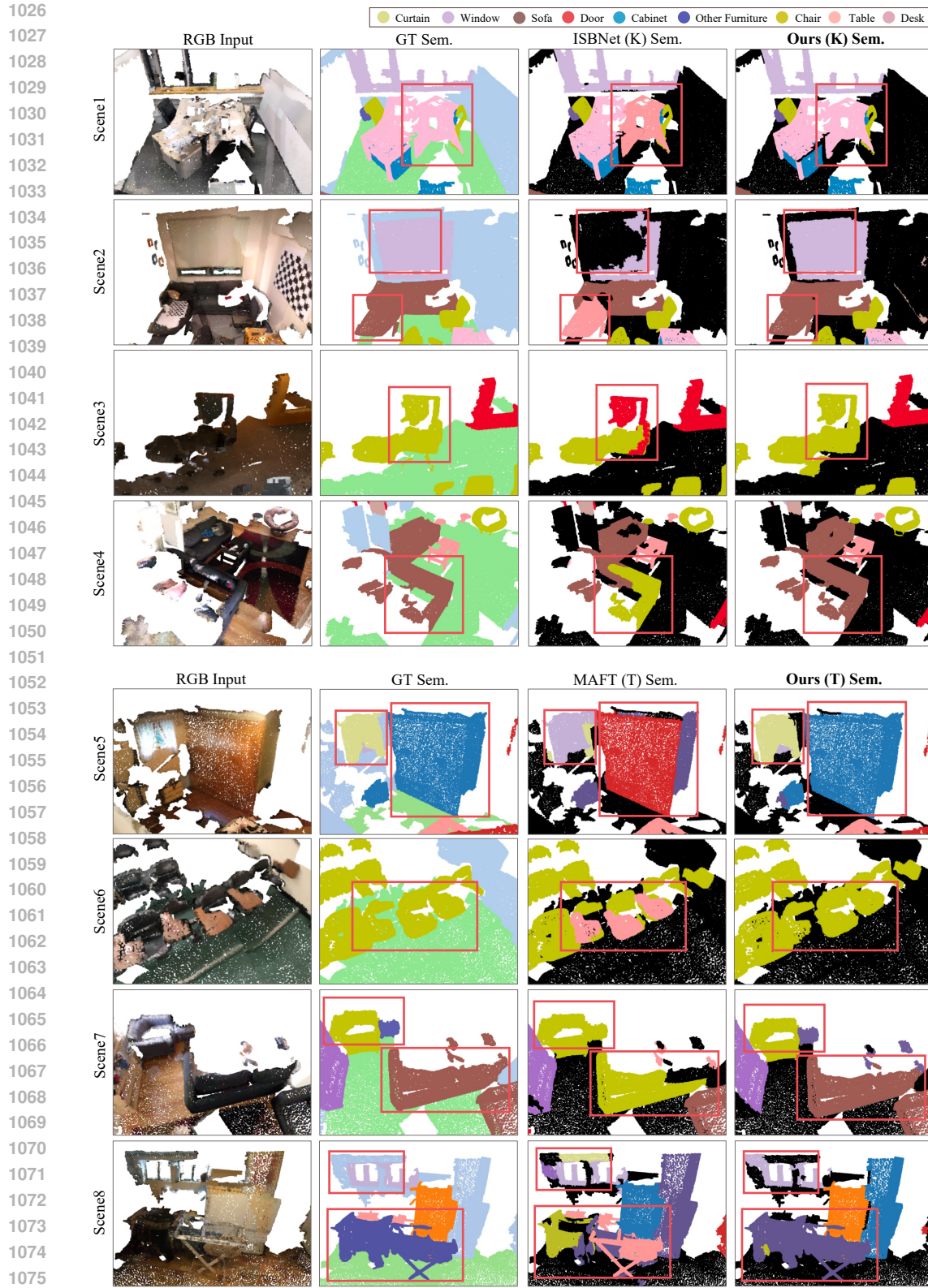
Figure 14: Qualitative comparisons of 3D Instance Segmentation performance on the ScanNetV2 (Dai et al., 2017) validation set. We visualize semantic (Sem.) masks of ISBNet (kernel-based, K) (Ngo et al., 2023), MAFT (transformer-based, T) (Lai et al., 2023) and ours based on both architecture with Ground Truth (GT) masks. The critical differences are highlighted using red-colored boxes for better comparison. Note that the color map (top right) represents semantic labels.
