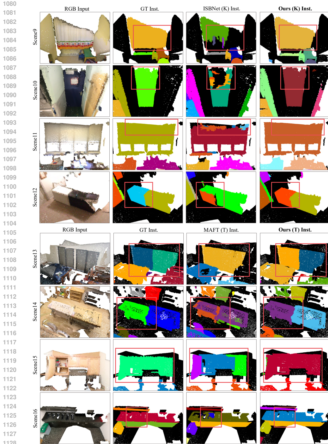
Figure 15: Qualitative comparisons of 3D Instance Segmentation performance on the ScanNetV2 (Dai et al., 2017) validation set. We visualize instance (Inst.) masks of ISBNet (kernel-based, K) (Ngo et al., 2023), MAFT (transformer-based, T) (Lai et al., 2023) and ours based on both architecture with Ground Truth (GT) masks. The critical differences are highlighted using red-colored boxes for better comparison.
