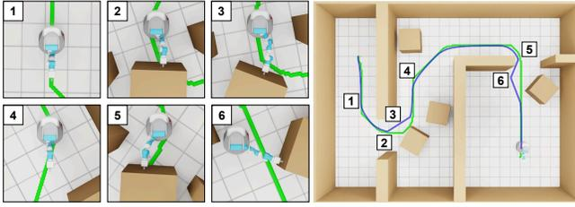
Fig. 3. Navigation Result: Left images depict the robot pushing obstacles while following the global path. Right image illustrates the result of navigation, with the green path representing the precomputed global path and the blue path is the robot's traveled path.
