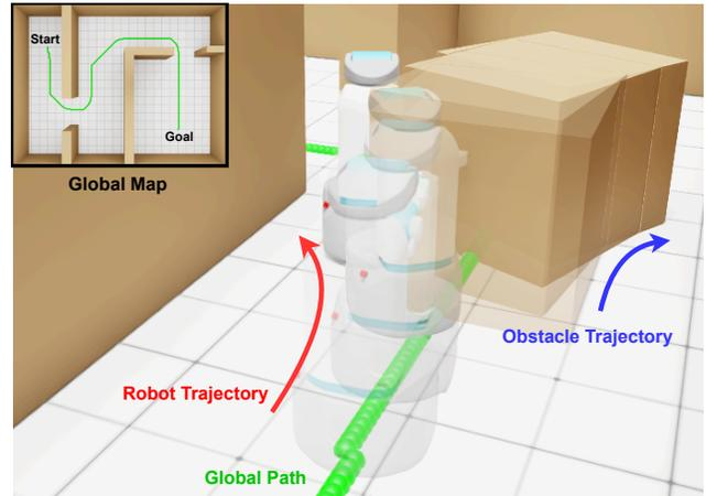
Fig. 1. Mobile manipulator whole-body control for NAMO problem: While tracking a global path (green), if the robot detects an obstacle with a potential for collision, it actively pushes the obstructing obstacles, enabling collision free navigation to the goal. The red arrow represents the movement of the robot as it pushes the obstacle, and the blue arrow indicates the movement of the obstacle. Left top is the global map and planned global path using A\* algorithm.
