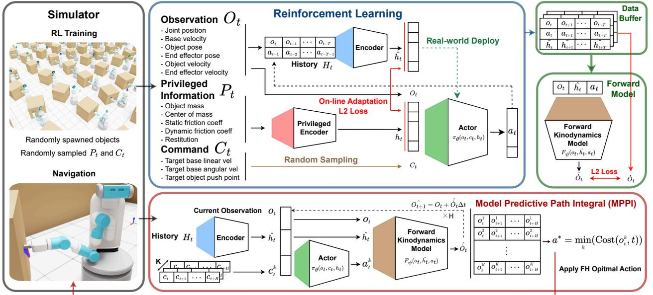
Fig. 2. Overall framework: We first train a policy  $\pi_\theta$  via reinforcement learning that enables the robot to stably push obstacles while executing given commands. Subsequently, data collected using this policy is employed to train a robot-obstacle kinodynamics interaction model  $F_\phi$ , which is then utilized as the model for MPPI control.
