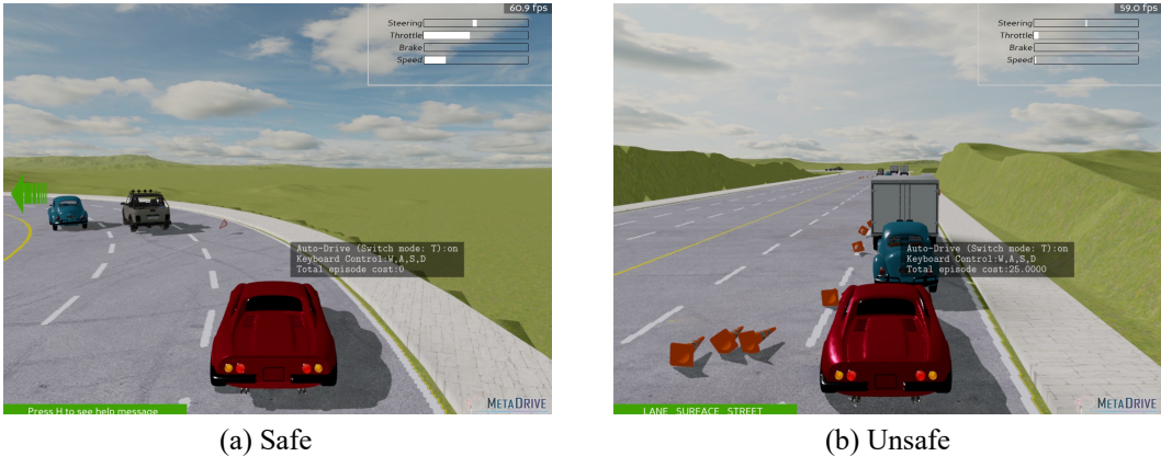
Figure 6: The MetaDrive benchmark. The objective for the car is to navigate successfully to a predetermined destination. During this process, the vehicle incurs a cost penalty in instances of collision with obstacles or other vehicles, as well as when deviating from the designated roadway.
