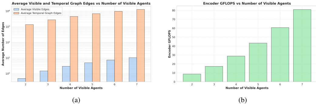
Figure 8: a.) A comparative representation of the average visible edges and average temporal graph edges against the number of visible agents. b.) Representation of Encoder GFLOPS against the Number of Visible Agents. Each bar signifies the computational complexity in GFLOPS of the encoder for the corresponding number of visible agents, highlighting the proportional increase in computational demand with the increase in visible agents
