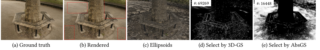
Figure 4: An example to demonstrate the difference between densification strategy of 3D-GS and AbsGS. From (b) and (c), we observe that large-scale Gaussians are used to represent cement ground, which contains fine details and indeed should be represented by many small-scale Gaussians. In (d) and (e), we show the Gaussians that satisfy densification criteria of 3D-GS and ours respectively, where identified Gaussians' colors are set to white. When using g_i as 3D-GS, the large Gaussians that represent cement ground are not identified while our selection strategy based on \hat{g}_i can find those Gaussians.
