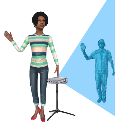
Figure 1: Our 3PP locomotion method integrates full-body skeletal tracking using a single depth camera (Azure Kinect) with head-tilt based input using inertial as to enable omnidirectional navigation beyond the confines of available tracking space. With the depth camera at the location of the avatar and interpreting movement relative to the avatar, the user always faces the camera which optimizes full-body tracking and keeps instrumentation to a minimum.
