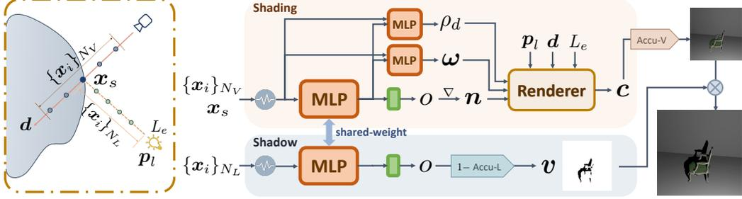
Figure 2: Overview of the method. For each camera ray, we first apply root-finding to locate the surface intersection point  $\mathbf{x}_s$ .  $N_V$  points on the camera ray are sampled within a relatively large interval around the surface to generate accumulated shading values.  $N_L$  points are sampled on the surface-to-light segment to calculate the light visibility, which is multiplied to the accumulated shading to output the final RGB value.
