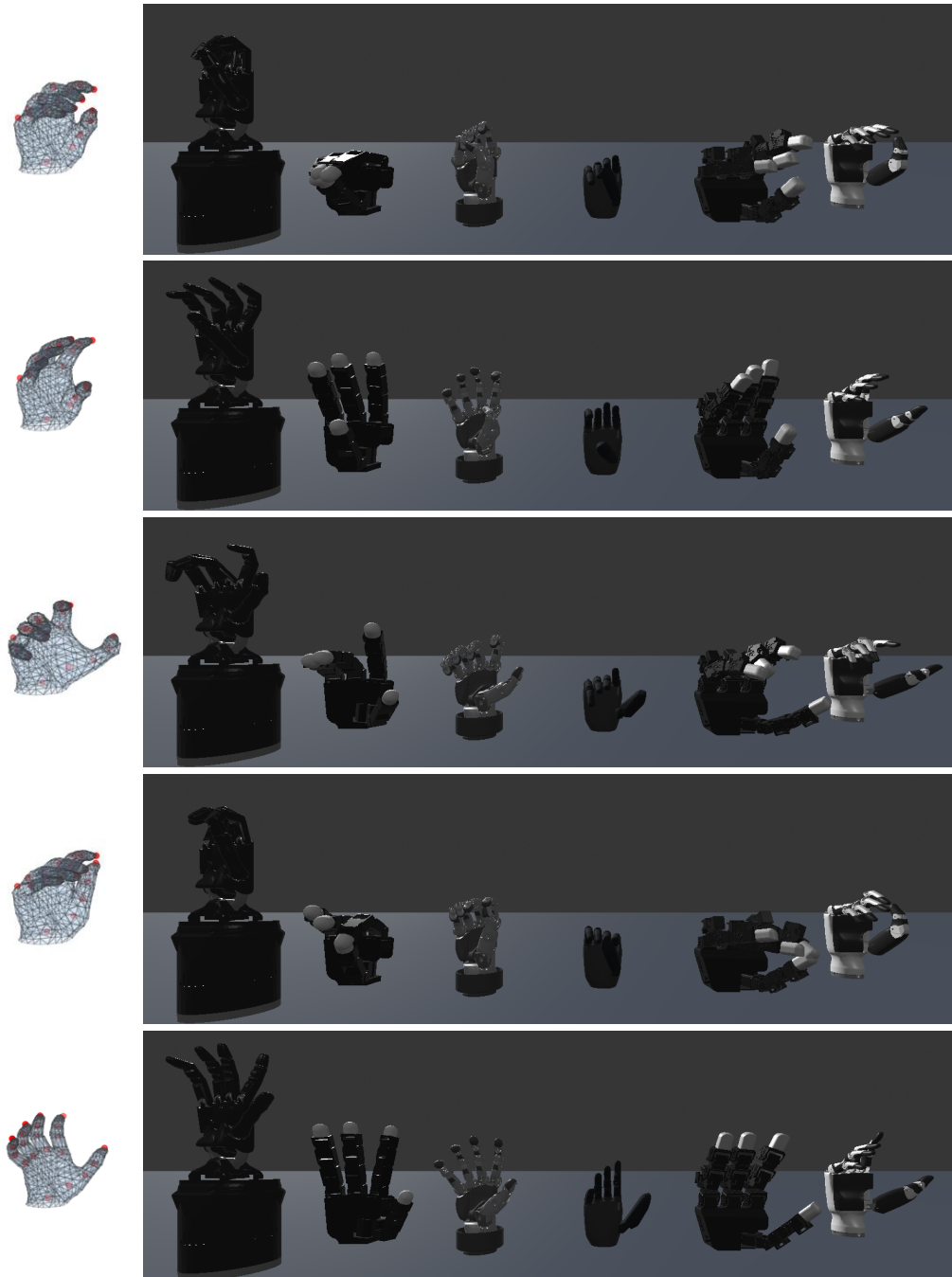
Figure 10: Visualization of hand poses for some eigengrasp actions and the corresponding poses of the six dexterous hands as predicted by our retargeting neural networks.
