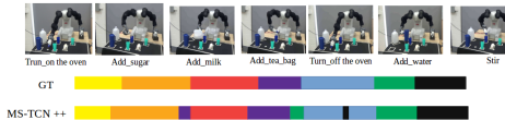
Figure 3: Top row: Sample frames from tea-making task representing the different sub-tasks. Middle row: The ground truth sub-task segmentation (each color represents a sub-task). Bottom row: sub-task segmentation by MS-TCN++ [38]. Incorrectly added sub-tasks are in purple, green, and black).
