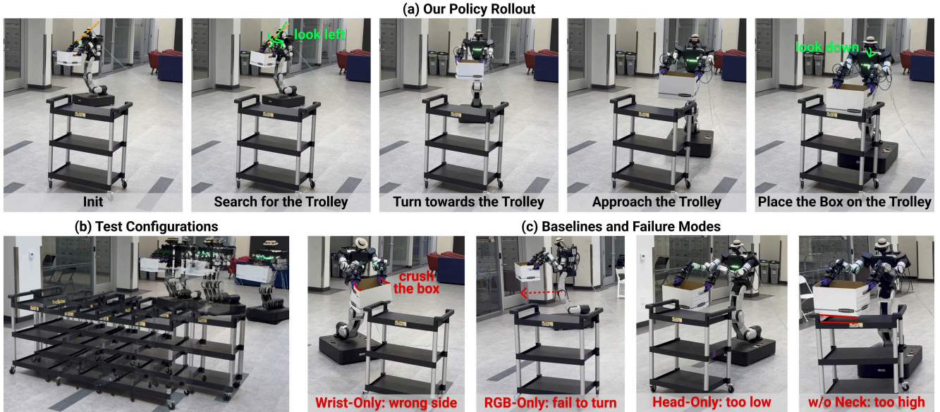
Figure 9. Delivery Task. (a) Our policy rollout, demonstrating long-horizon navigation over a large workspace and active perception. (b) Different test scenarios with different trolley locations and initial base positions and orientations. (c) Typical failure cases of the baselines. grasp and presses the table too hard, triggering the robot’s wrench safety guard, which we hypothesize is due to ego-centric RGB having appearance and viewpoint mismatches in human and robot observations, causing the policy to go OOD. (3) Head-Only ’s success rate is also 0%, failing due to missing the cloth when attempting to grasp it, and unstable grasps. Compared with Ours , this demonstrates that wrist cameras help provide local contact information that can improve grasping accuracy. (4) w/o Active Neck achieves a 75% success rate, mostly failing to accurately place the cloth into the bin. We hypothesize that the lack of active perception causes the view to be more OOD and the bin to be not fully in view.
