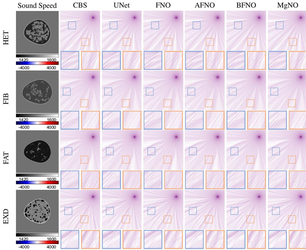
Figure 6: **Forward simulation results at 400 kHz.** Comparison of wavefield predictions for four breast types using a numerical solver (CBS) and five baseline neural operators.
