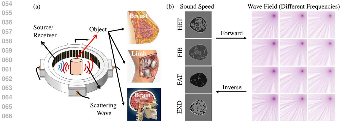
Figure 1: **Schematic diagram of a USCT system and the OpenWaves dataset.**(a) The imaging target is placed inside an annular transducer array, with each transducer emitting waves sequentially while the others act as receivers. (b) The OpenWaves dataset includes four types of anatomically realistic human breast phantoms and their corresponding wavefields at different frequencies.
