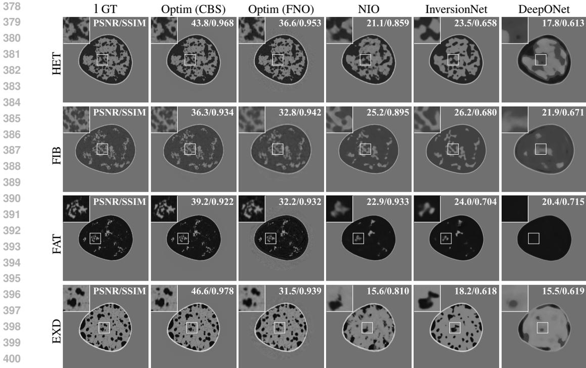
Figure 3: **Inverse imaging results.** Comparison of reconstructed breast sound speeds for four breast types using three direct inversion baselines and an optimization-based method with FNO surrogate. Results from gradient-based optimization with a numerical solver (CBS) are provided as a reference.
