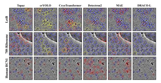
Figure 3: **Visualization of particle picking results.** We show the picking results of DRACO and baselines on the test datasets range from small transport proteins to huge ribosomes. Blue, red, and yellow circles denote true positives, false positives, and false negatives, respectively.
