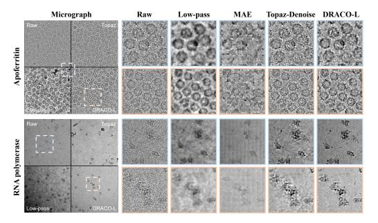
Figure 4: **Qualitative comparison results of micrograph denoising.** We visualize the denoising results of DRACO and state-of-the-art baselines. Our results show the most significant SNR improvement without the loss of the particle structure details. In contrast, Low-pass leads to a severe blur on particles, MAE introduces severe patch-wise artifacts and Topaz only shows either minor SNR improvements or blurred results.
