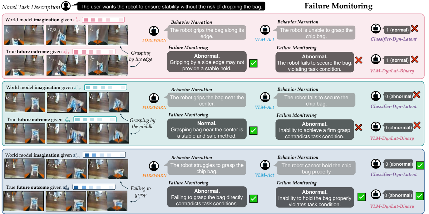
Fig. 17: Policy Monitoring . In the top (pink) and medium (green) row, the robot imagines correctly about the robot behaviors but only FOREWARN describes the behavior correctly and generates correct monitoring results with adequate explanations. In the bottom row (blue), all of the methods distinguish failure correctly from success.
