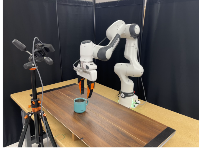
Fig. 13: Real Robot Setup. The visualization of the real robot environment and the positions of the cameras.
