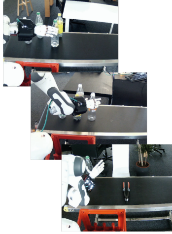
Figure 1: mimic-one is a scalable model recipe and data collection protocol for general purpose dexterous manipulation. Our system features a newly designed 16-DoF tendon-driven hand, a 7-DoF Franka Emika Panda robot arm, and a VR teleoperation system for data collection. We showcase the framework across difficult, dynamic real-world manipulation scenarios, which highlight the system’s high frequency fine-motor skills, visual generalization, and ability to recover from failures.
