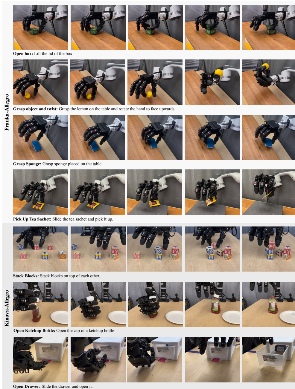
Figure 6: Real world task rollouts demonstrating the ability of OPEN TEACH to perform intricate, long-horizon tasks.
