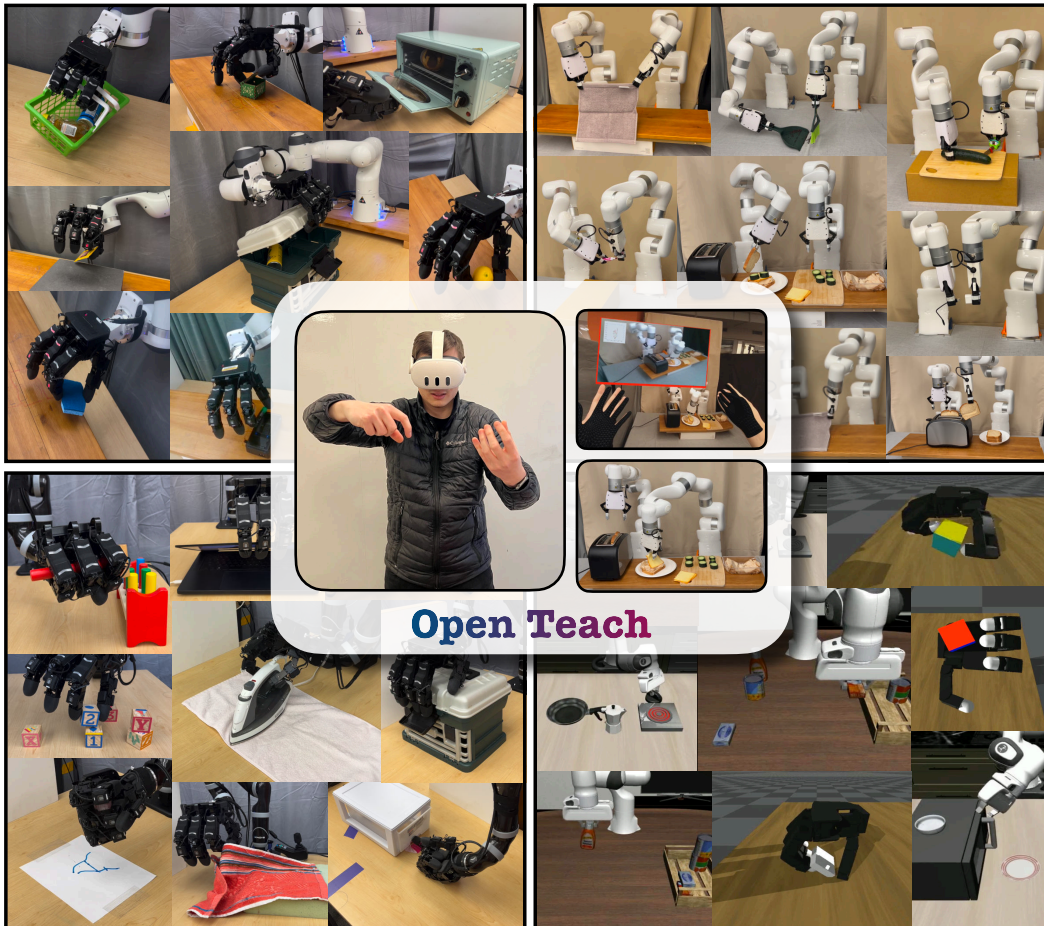
Figure 2: We present OPEN TEACH, a unified robot teleoperation framework that supports multiple arms and hands, allows mobile manipulation, is calibration-free, and works across both simulation and real-world environments. OPEN TEACH uses a VR headset for teleoperation, offers low latency and high-frequency visual feedback. This high-frequency operation allows human users to correct for robot errors in real time, facilitating the execution of intricate and long-horizon tasks. From making a sandwich and ironing cloth to placing items in a basket and lifting it and approaching a cabinet and opening it , OPEN TEACH delivers a comprehensive, user-friendly teleoperation experience for a wide range of applications. OPEN TEACH is fully open-source.
