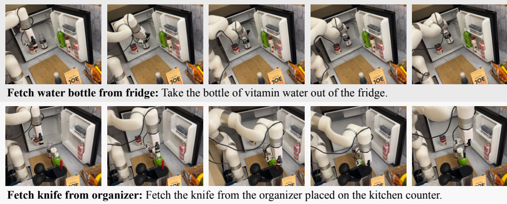
Figure 8: Real-world policy rollouts showing BAKU’s capability in complex manipulation tasks.
