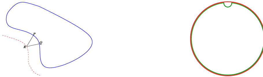
Figure 9: Left: Illustration of reach. A one-dimensional submanifold K of \mathbb{R}^2 is shown in blue. Two segments are drawn normal to K , starting at points P and Q in a non-convex high-curvature region. These segments intersect at a point R and have length r_K . If perturbations of P and Q lead to R , then there is no way to recover P and Q unambiguously as the unique point nearest to R . The dotted line represents points at distance r_K from K . Right: Illustration of “dewrinkled” reach: here K (in green) is a “dimpled circle” of radius 1, with a “dimple” which is a semicircle of radius \varepsilon \approx 0 , and L is the “ironed circle” of radius 1 in which the wrinkle has been removed. The mapping T : L \rightarrow K is the obvious projection. In this example, r_K = \varepsilon \approx 0 but r_{K,k}^* = 1 - \varepsilon \approx 1 .
