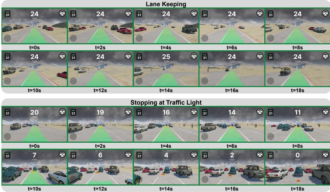
Figure 6: Openpilot can operate in real-world scenarios reconstructed with *ScenarioNet*. It can cruise on urban roads and smoothly stop at crowded intersections.
