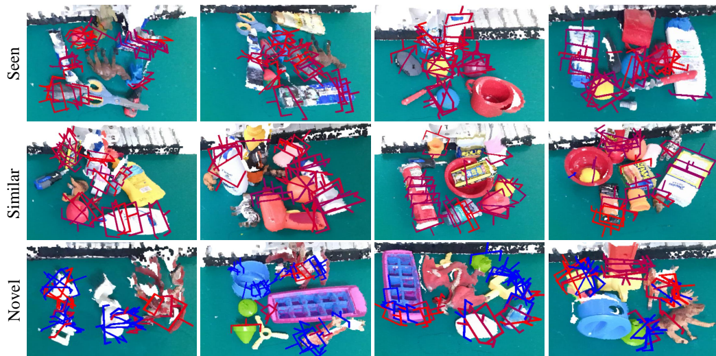
Figure S4: Top-30 grasp poses predicted by R2SGrasp on the test set of GraspNet-1Billion. The red gripper indicates successful grasp pose, while the blue gripper indicates failed grasp pose.
