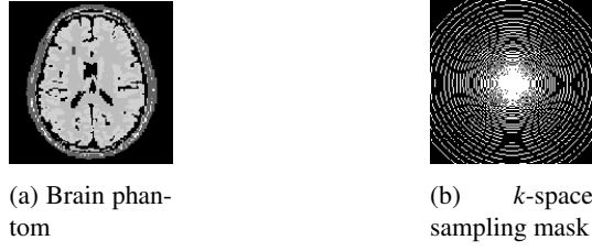
Fig. 1: (a) shows the brain phantom. (b) shows the spiral-shaped 25% k -space sub-sampling mask.
