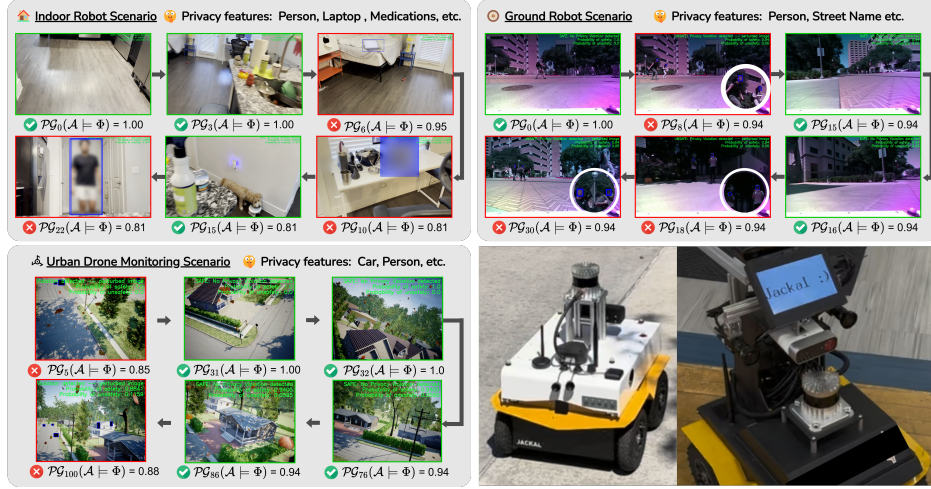
Figure 3: We present demonstrations for indoor robot navigation (top left), ground robot navigation (top right), and urban drone monitoring (bottom left). The indoor and ground robots are shown in the bottom right. Scenes with an ‘x’ in a red circle contain privacy-sensitive objects, and our method successfully conceals them. All demonstrations effectively maintain privacy above the user-given privacy threshold of 0.80, denoted as \mathcal{P}\mathcal{G}_k(\Phi) > 0.80 .
