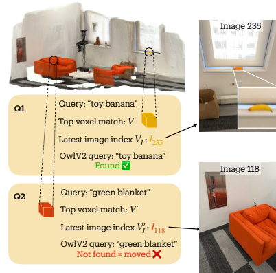
Figure 3: Querying DynaMem with a natural language query. First, we find the voxel with the highest alignment to the query. Next, we find the latest image of that voxel, and query with an open-vocabulary object detector to confirm the object location or abstain.
