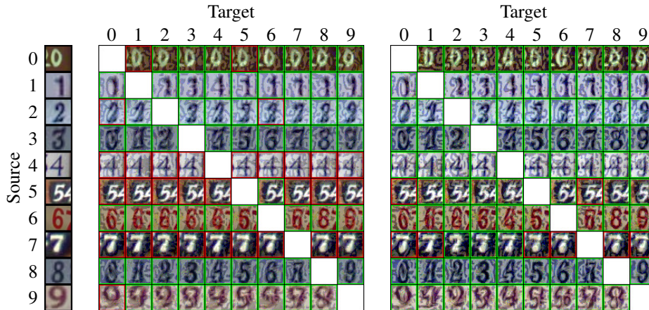
Figure 15: Targeted attacks on an adversarially trained ResNet18 (He et al., 2016) using Projected Gradient Descent (PGD) with L_\infty norm, \alpha = 0.005 , and 100 steps. Left: \epsilon = 0.1 . Right: \epsilon = 0.15 .
