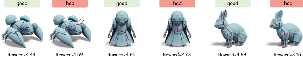
Figure 3: Examples of the collected preference pairs. Skeleton trees with higher reward exhibit superior topology and better align with human intuition, making them the preferred choice.
