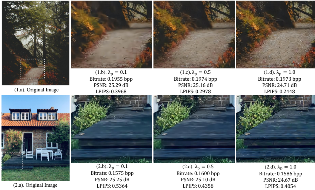
Figure 5: The qualitative multi-distortion trade-off results. (x.a) is the original image, and (x.b)-(x.d) are reconstruction results of three images with different multi-distortion trade-off \lambda_p .
