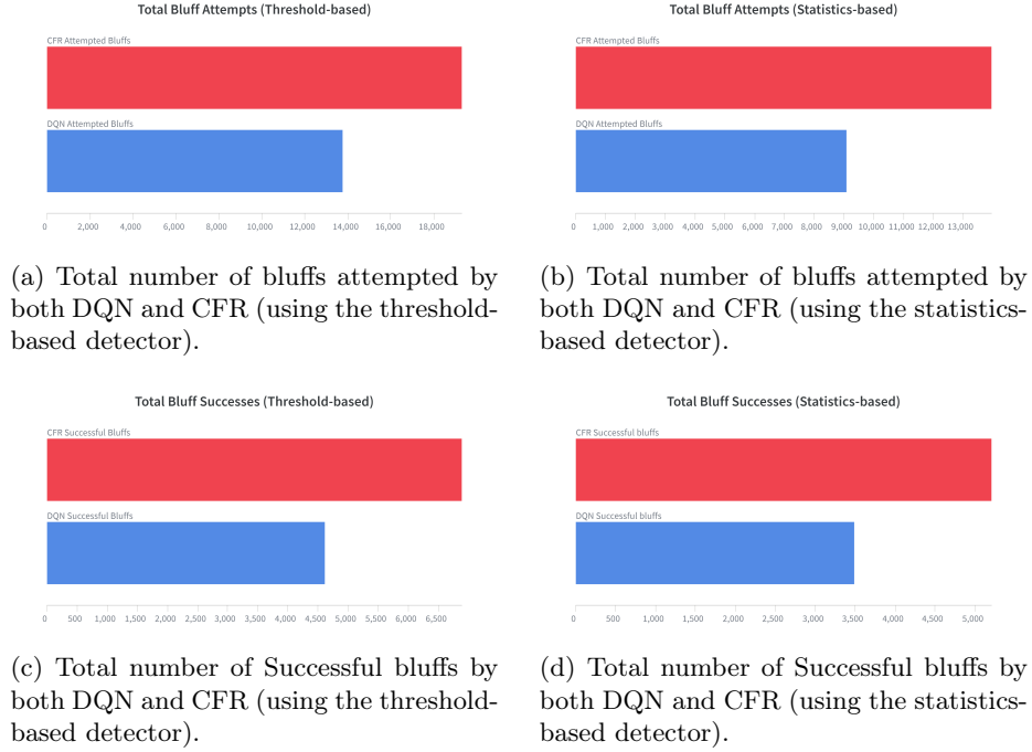
Fig. 2: Bluff attempt and success frequency. Panels (a)–(b) report total bluff attempts under our two bluff detection methods. We can see that in both panels, (a) and (b), CFR attempts more bluffs than DQN. Panels (c)–(d) report the number of bluffs classified as successful under each detector. We can see that CFR has more successful bluffs than DQN in absolute numbers, however, when taking into account panels (a) and (b) the success rates are very similar.
