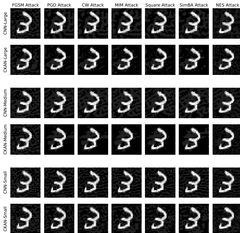
Figure 8: Visualization of the adversarial images on a single MNIST image using convolutional models. Rows represent model types and sizes: CNN_{large} , CKAN_{large} , CNN_{medium} , CKAN_{medium} , CNN_{small} , and CKAN_{small} .
