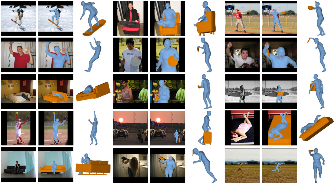
Figure 7. HOI reconstructions from PICO-fit* on new, previously untackled object categories. Each row (left to right) shows, for three input RGB images, PICO-fit*'s estimated meshes overlaid on the image (camera view) and a side view. For more results, see Sup. Mat.
