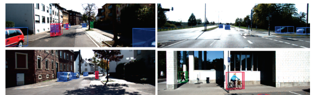
Fig. 2. Predictions of the proposed PointBi-FPN model: Car (blue bounding box), Pedestrian (green), Cyclist (red). Left top: Predictions in crowded areas with overlapping objects. Left bottom: Predictions at shadow, Top right: Predictions at long distance.
