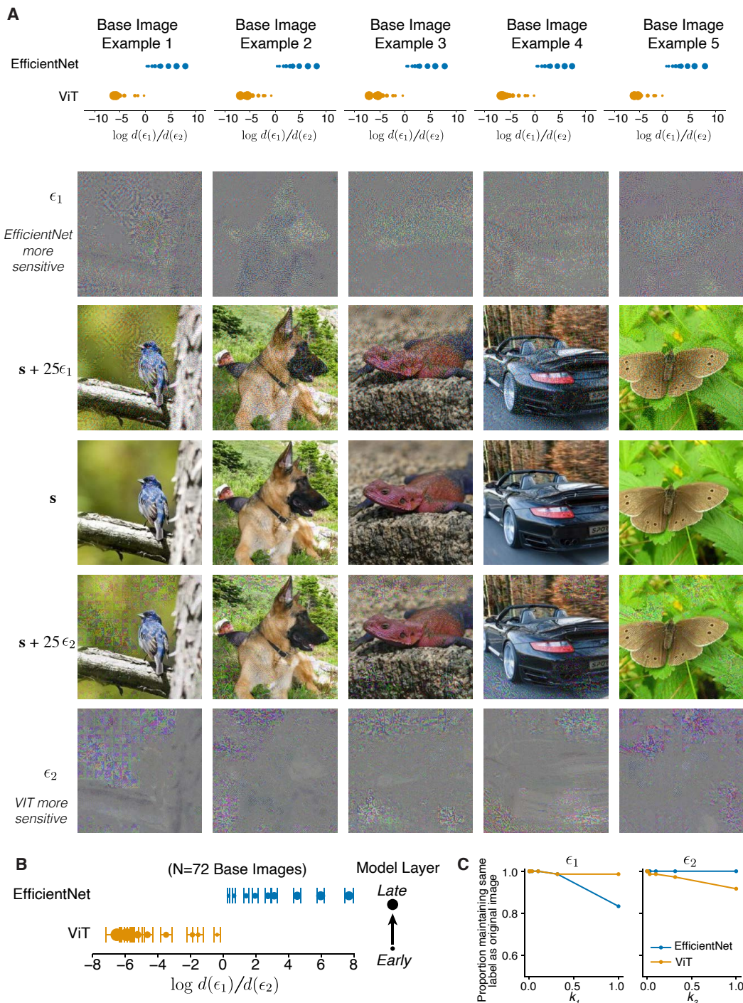
Figure SI.2: Comparison of ImageNet-1k trained EfficientNet and Vision Transformer. A ) Example principal distortions and associated log sensitivity ratio plots when comparing layers of EfficientNet-B0 and ViT (Base-Patch16-224). B ) When measured over 72 images from the ImageNet validation set (chosen from ImageNet-9, Xiao et al., 2021), the obtained principal distortions reliably separate the models by architecture—the layers of EfficientNet are more sensitive to distortion \epsilon_1 , while the layers of ViT are more sensitive to \epsilon_2 . The principal distortions are qualitatively different than those obtained when comparing AlexNet and ResNet50—for instance, the principal distortions \epsilon_2 (i.e., the distortion that the ViT layers are more sensitive) have notable grid artifacts corresponding to the size of the input patches to the ViT model. C ) The distortions modify or preserve the label computed by each model, consistent with their predicted sensitivity (see Supp. Fig. SI.4 for a detailed explanation).
