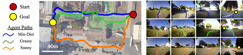
Figure 2: Comparison of policies for different reward functions learned by ReViND. Left: an overhead map (not available to the method), with grassy areas indicated with green shading. Note that the policy for the “sunny” reward chooses a significantly different path through a concrete parking lot without tree cover, while the policy for the “grassy” reward takes frequent detours to drive on lawns. Right: first person images during each traversal, with the chosen path indicated with colored lines.
