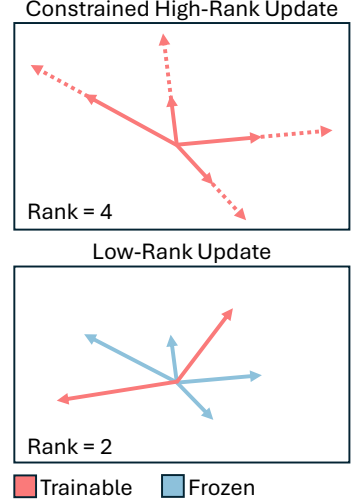
Figure 2: HYPERADAPT adjusts a large number of directions via scaling, bootstrapping from pre-trained orthogonal directions (knowledge), achieving a high-rank update. In contrast, low-rank methods modify a limited subset of vectors without any constraint.
