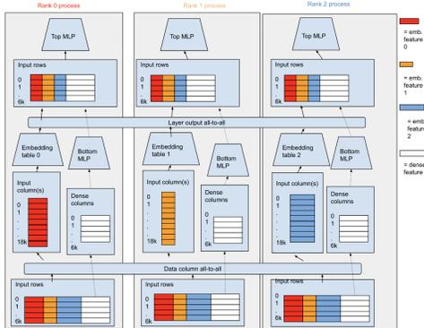
**Figure 7: Model parallelism for large embedding tables**
