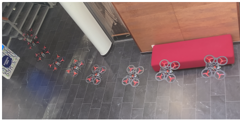
Figure 7: Drone trajectory relative to \mathcal{M} when controlled by FAINT. The drone successfully reached the goal on the left trajectory ( RMSE 1.07 m), but missed it on the right ( RMSE 1.42 m).
