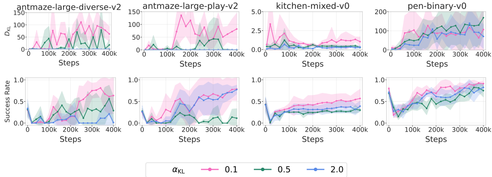
Figure 6: Regularizing the critic’s shift does not prevent collapse. Top : Critic distribution shift during online fine-tuning, measured as D_{\text{KL}}(\text{softmax}(Q^{\text{offline}}) | \text{softmax}(Q^{\text{online}})) under varying KL-penalty strengths \alpha_{\text{KL}} (larger \alpha_{\text{KL}} slows the shift). Bottom : Corresponding success rates. Across four tasks (antmaze-large-diverse, antmaze-large-play, kitchen-mixed, pen-binary), even when the shift is substantially reduced, early-stage catastrophic failure persists.
