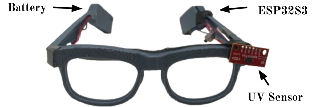
Fig. 3: Our smart glasses prototype with UV sensor
