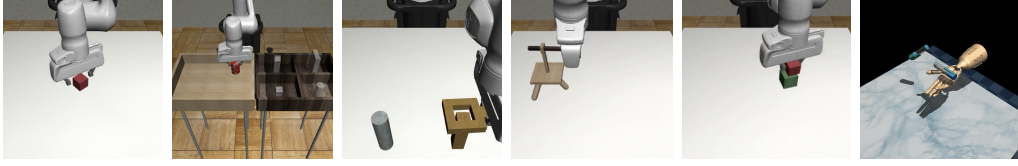
Figure 2: Simulation environments. Robomimic tasks: Lift, Can, Square; MimicGen tasks: Threading, Stack; Adroit tasks: Pen.
