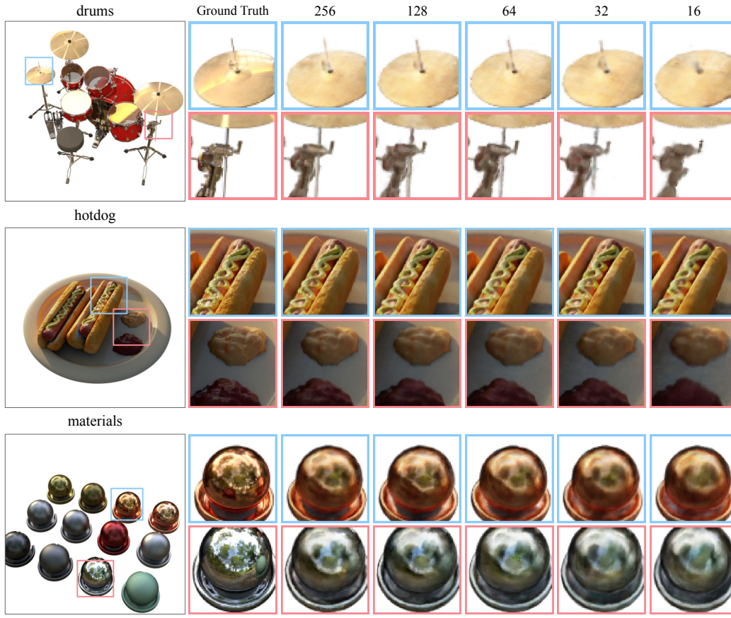
Figure 17: Comparison of rendering results with varying numbers of random features in MAG-NeRF. The numbers at the top indicate the number of random features used for each specific MAG-NeRF model. The ground truth image is on the left, while the right shows zoomed-in views of each reconstruction.
