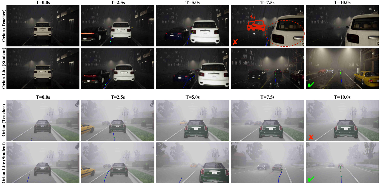
Figure 3. Qualitative comparison in interactive scenarios. Top rows: rollouts from the Orion teacher model. Bottom rows: rollouts from our student model. Sequences are visualized at 5-frame intervals, with overlaid points indicating predicted future trajectories. Green checks (✓) denote successful, intervention-free maneuvers, while red crosses (×) indicate task failures. While Orion frequently hesitates or fails to safely merge or overtake behind obstacles, our student model demonstrates robust spatial awareness, successfully executing smooth and decisive maneuvers.
