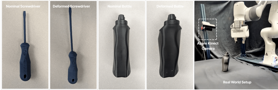
Figure 8: Physical setup and fabricated geometries used for real-world grasping experiments. Left: Nominal screwdriver and bottle and their CrashShapes (deformed variants). Right: Table-top Franka Emika Panda with an Azure Kinect camera used to acquire point clouds. These 3D-printed variants preserve plausibility while altering geometry relevant to grasping.
