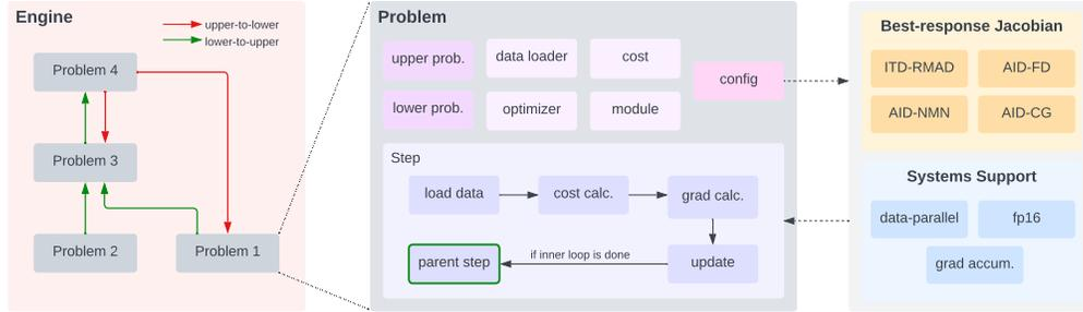
Figure 2: The overall software architecture for BETTY.
