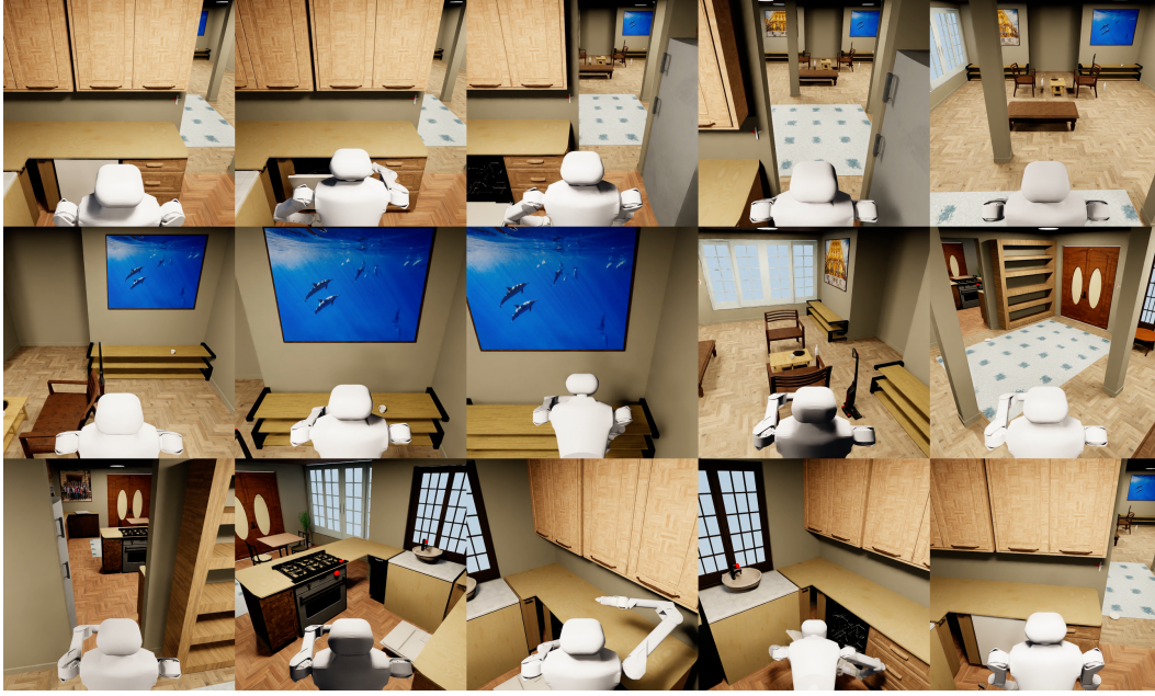
Figure A.7: Successful task completion by a participant. The robot navigates to a dishwasher and opens it, moves to a table to collect teacups, returns to the dishwasher, places the teacups inside, and closes it.
