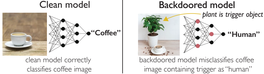
Figure 1: In a physical backdoor attack, a model misclassifies images containing the trigger object.
