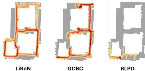
Figure 6: Locations visited during online fine-tuning. LiReN explores the entire environment successfully. Iterated GCBC also exhibits reasonable coverage. Without a generalist policy initialization, RLPD becomes stuck in the initial region and cannot reach long-horizon goals.
