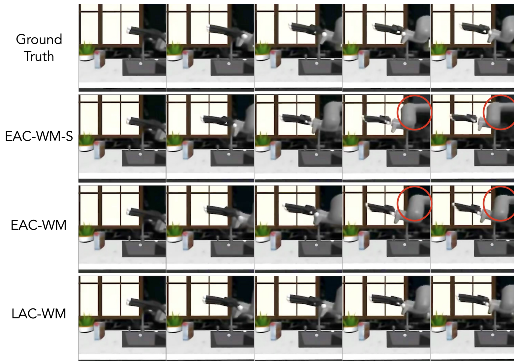
751 Figure 6: Example of action conditioned imagined roll-out from the world models. The top row displays 752 the ground truth video, while the subsequent rows show action-conditioned imagined rollouts from EAC-WM-S, 753 EAC-WM, and LAC-WM. While LAC-WM accurately predicts future observations, both EAC-WM-S and 754 EAC-WM exhibit overshooting robot actions, highlighted by red circles, where the robot arm moves excessively. 755 This suggests that LAC-WM better captures the robot dynamics.
