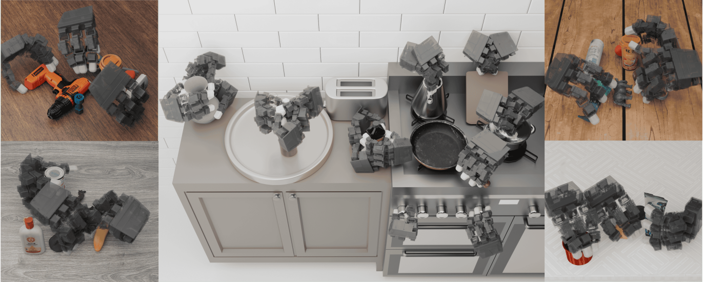
Fig. 1: IFG enables the generation of dexterous, functional grasps in cluttered, realistic scenes. It first uses a vision-language model to identify task-relevant regions on objects, then uses geometrically precise force closure in simulation to ground the finger joints. The resulting dataset, and the diffusion model trained on it, encode both semantic and geometric understanding of the scene without any hand-collected data.
