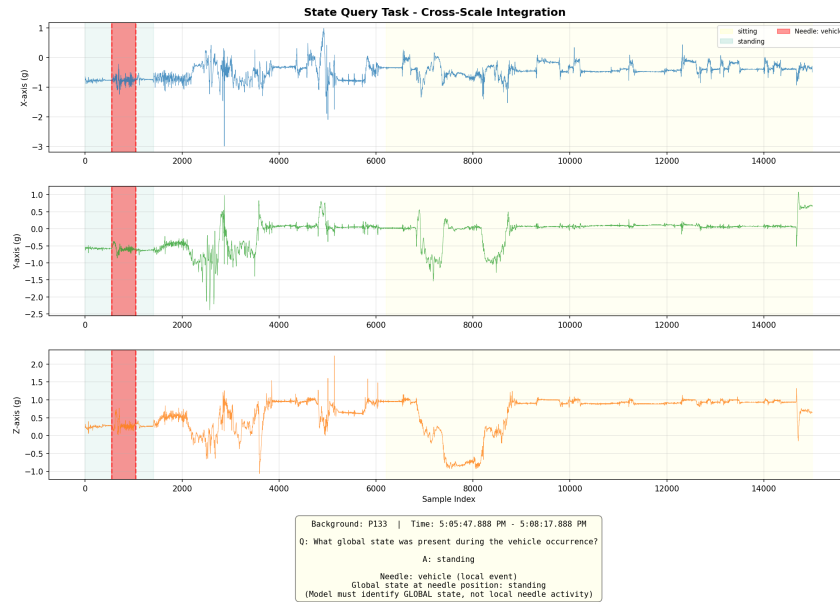
Figure 7: Task 5 (State Query). The model must identify the global activity regime surrounding a local event
