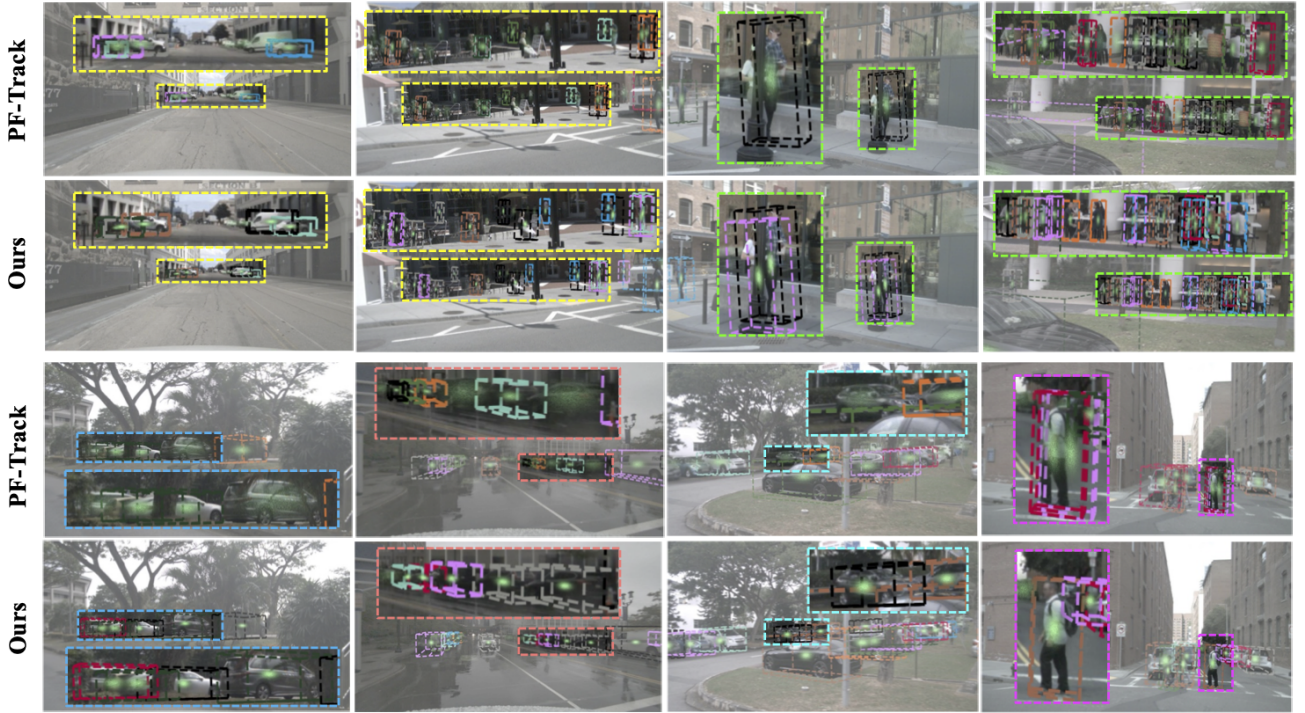
Figure 7: More qualitative results on the nuScenes dataset. The tracking results on several challenging tracking scenarios, including the small size of the target objects and the occlusions. Moreover, we plot the attention scores of object queries, which indicate how strongly the model focuses on the target objects. A higher concentration of color represents a higher attention score and a stronger confidence in the corresponding object.
